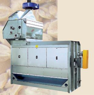
As well as separating good quality grain from splits and trash, this rotary drum removes them completely. The rotary drum cleaner with aspiration is essential for cleaning cereals that have to be stocked for a long time (avoiding overheating, which can be caused by chaff, husks, split grains etc.). The final product will be healthier and have a pleasant aspect.
