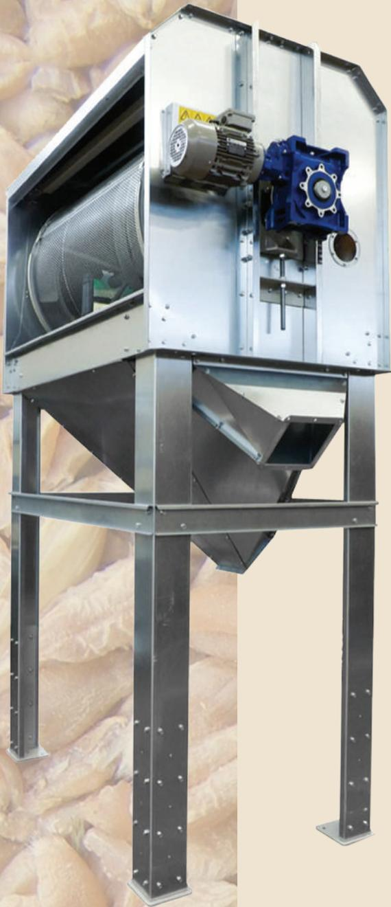
This pre-cleaner is designed for fast removal of light and rough impurities in cereal. It is essential for the quality of cereal that a pre-cleaner is installed at the drier inlet. It homogenises the product, preventing clogging and reducing energy consumption. The version with aspiration reduces the emission of dust into the atmosphere.
