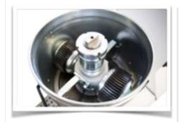
miniPelleter is put on the rigid frame with reinforcement plates for a solid gear and a driving engine 15 or 18.5 kW.
