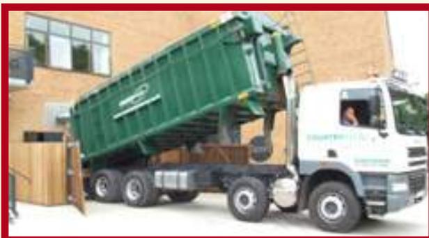
If the space is not adequate for a delivery to be made then the only solution is to move the delivery space, but this in its self can cause further issues. The decision will then need to be made as to whether you move the boiler along with the woodchip store or bunker, and then pipe the heat to where
