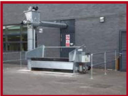
One particular client put a woodchip blower system in place that was producing about 120db of noise. During the early periods of operation local residents complained about the noise and dust generated during delivery. Eventually the client had to replace the system with a Perry Biomass handling BIO Intake which reduced the noise generated during the delivery to less than 60db.
